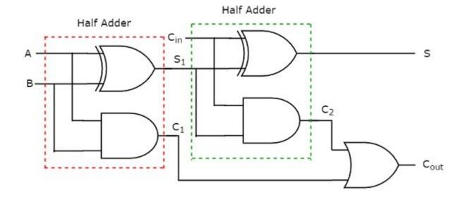
This adder is called as **Full adder** because for implementing one Full adder, we require two Half adders and one OR gate. If C<sub>in</sub> is zero, then Full adder becomes Half adder. We can verify it easily from the above circuit diagram or from the Boolean functions of outputs of Full adder.
