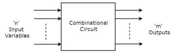
This combinational circuit has 'n' input variables and 'm' outputs. Each combination of input variables will affect the outputss.
