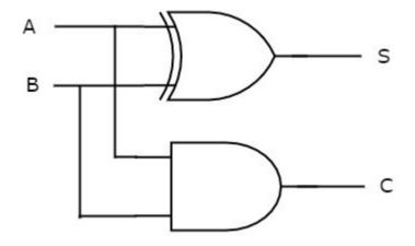
In the above circuit, a two input Ex-OR gate & two input AND gate produces sum, S & carry, C respectively. Therefore, Half-adder performs the addition of two bits.
