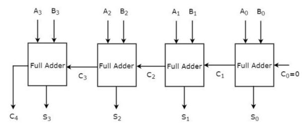
Here, the 4 Full adders are cascaded. Each Full adder is getting the respective bits of two parallel inputs A & B. The carry output of one Full adder will be the carry input of subsequent higher order Full adder. This 4-bit binary adder produces the resultant sum having at most 5 bits. So, carry out of last stage Full adder will be the MSB.
